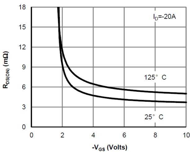
Figure 5: On-Resistance vs. Gate-Source Voltage (Note E)
