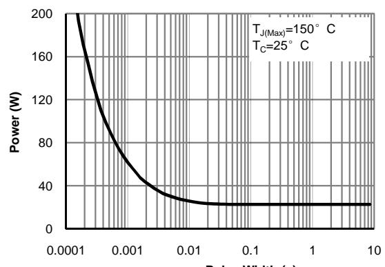
Figure 10: Single Pulse Power Rating Junction-to-Cooling-Circuit (Note F)
