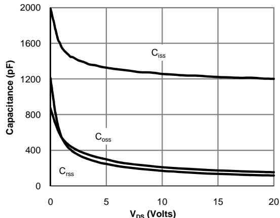
Figure 8: Capacitance Characteristics
